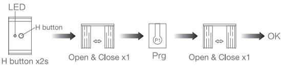
Remove controller B via pre-existing controller A
