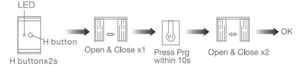
Way 3: Power on, add controller B via pre-existing controller A
